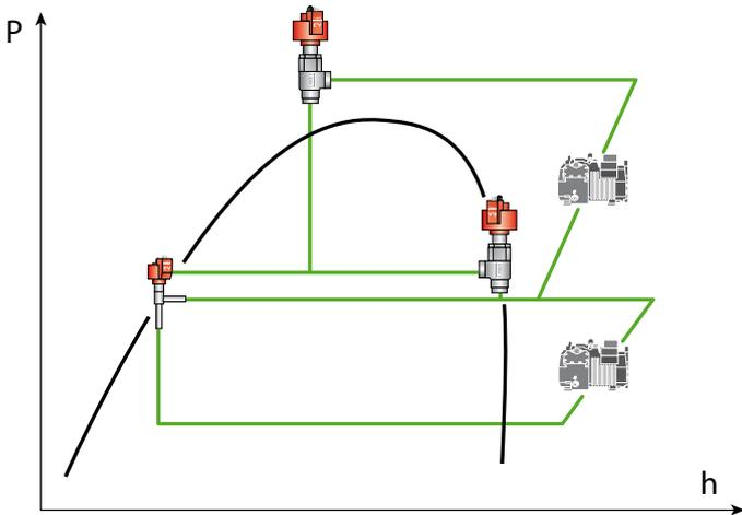
The HPV valve control algorithm on pRack pR300T is managed based on the gas cooler outlet temperature T<sub>GC</sub> and gas cooler pressure P<sub>GC</sub>. Depending on operating conditions, the system can work in:
