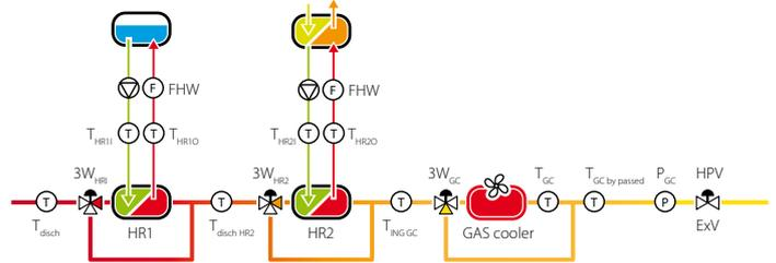
Heat recovery management allows complete control of two heat exchangers and related circulating pumps (in the case of CO<sub>2</sub>-water). Activation and control of each heat recovery cycle is based on the percentage of heat demand, calculated using one of the following:
