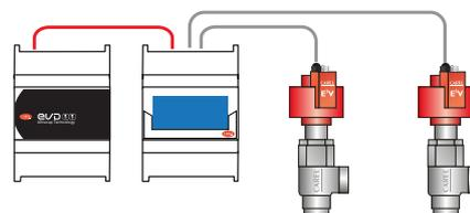
**MPXPRO & E2V: controller for multiplexed showcases and stepper electronic expansion valve.**
