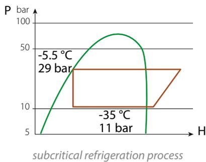
The primary cycle is managed using a traditional refrigerant, with the task of keeping condensing temperature for the CO<sub>2</sub> cycle below the critical point, generally between -5 and -10 °C.
