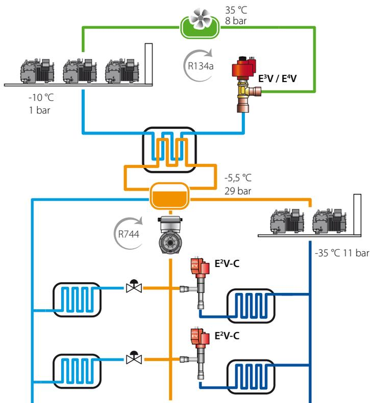
example of pumped subcritical CO<sub>2</sub> system
