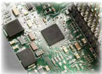
Carel has developed a proprietary chip using ASIC technology (Application-Specific Integrated Circuit), ensuring greater system flexibility as manufacturers can use the same size board for different applications.
